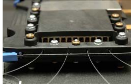
Fiber optic sensors protruding from a fuel cell power assembly prior to testing for moisture content fluctuations during high power operation.
