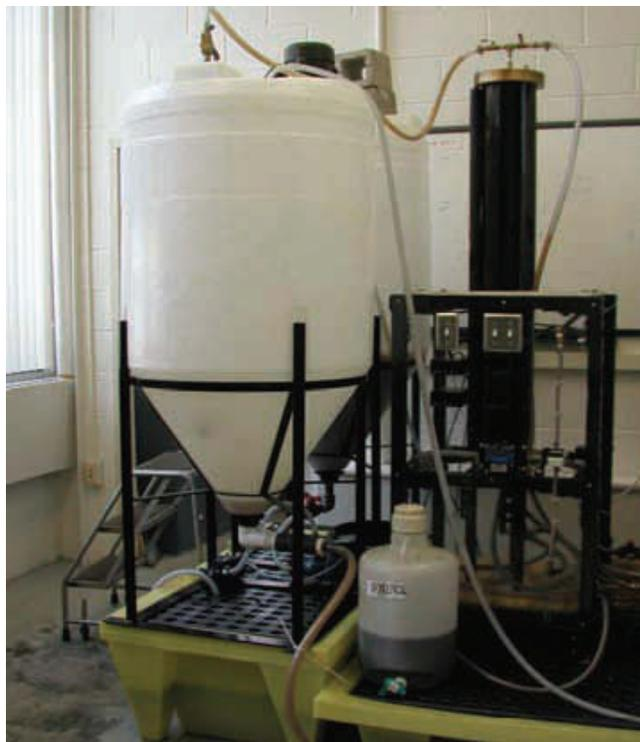
grease, a commercial waste vegetable oil, for the demonstration. In the week preceding the continuous run, Mr. Boucher pretreated the waste cooking oil to neutralize and remove free fatty acids and contaminants that resulted from the oil's earlier use in food production.
