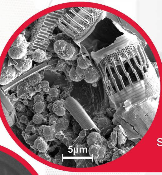
Titanium oxide spheres mixed with diatom skeletons.
