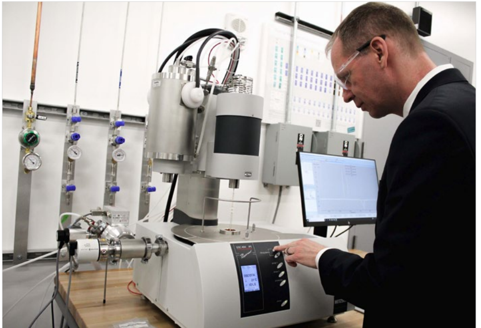
Hebert works with equipment to determine melting points and other thermodynamic properties at temperatures up to about 3,000 degrees Fahrenheit. (Carson Stifel/UConn Photo)
