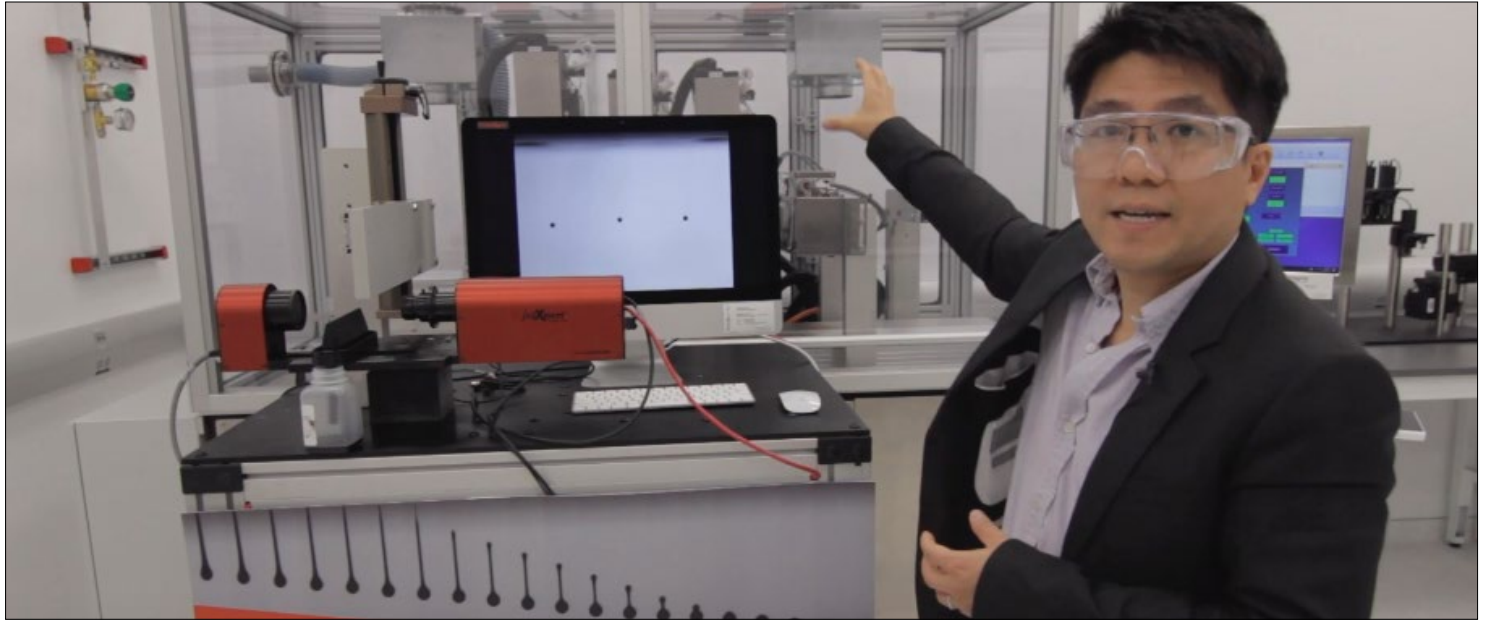
Chemical Engineering Professor Anson Ma explains the "drop watcher system" on HuskyJet, which gives the user the ability to test and measure the droplet volume, velocity, and trajectory of any new ink or substance to achieve optimal printing performance.
