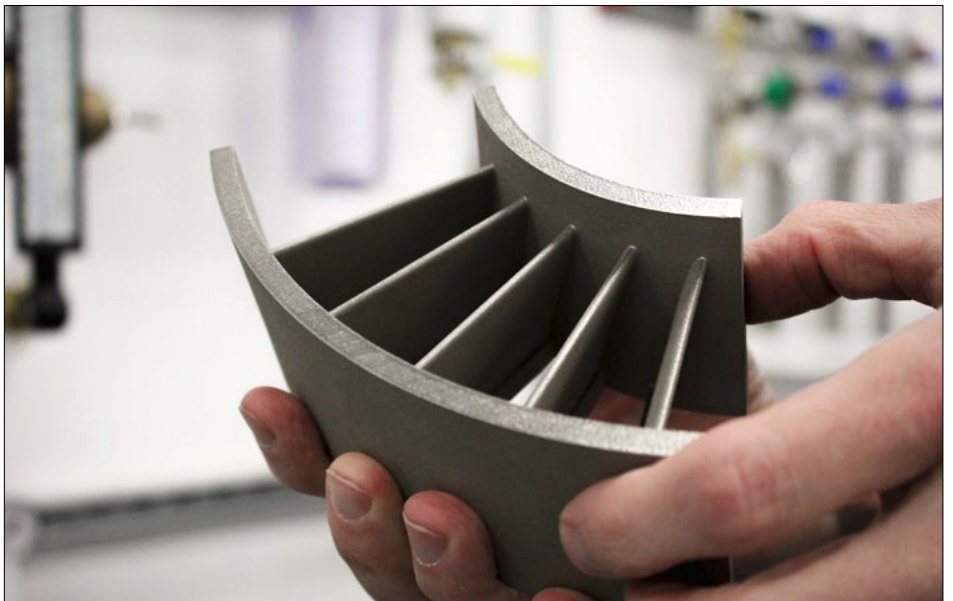
Hebert holds additively manufactured samples for R&D that emulate real-world component designs. (Carson Stifel/UConn Photo)
