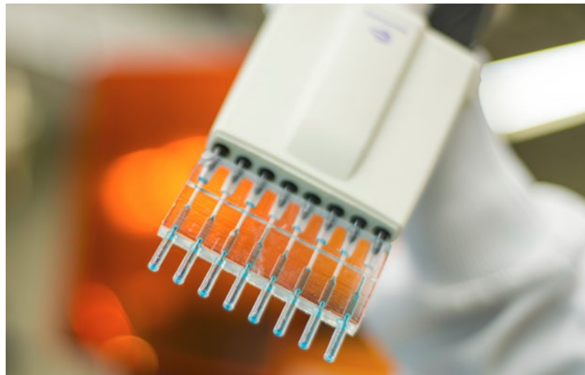
Mohamed Sharafeldin, holds a unique pipette tip created with a 3D printer. (Sean Flynn/UConn Photo)
